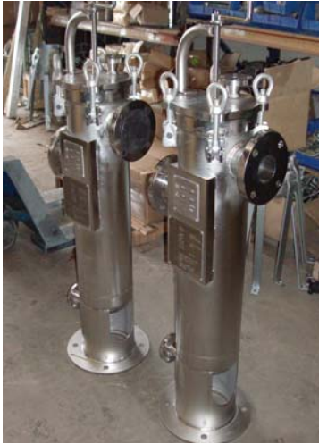
Above: Newly fabricated and hydro-tested single-round housings await crating.
