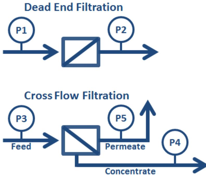
Figure 7 In this figure, the differential pressure for the dead end filtration system is  $P1-P2$ . The differential pressure for the cross flow filtration is  $P4-P3$ . The Trans-Membrane-Pressure (TMP) for the cross flow filtrations system is  $(P3+P4)/2 - P5$ .
