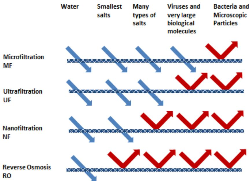
Figure 6 MF, UF, NF, and RO membranes differ in what they allow to filter through, and what they “reject”. Rejected species are represented by bent (red) arrows, while species that filter through the membrane are represented by straight (blue) arrows. Note that RO removes the tiniest salts, and that removal of nanometer-scale viruses is not nanofiltration (NF) but instead is called ultrafiltration (UF). The arrows are not meant to indicate 100% of anything, but represent the general result.
