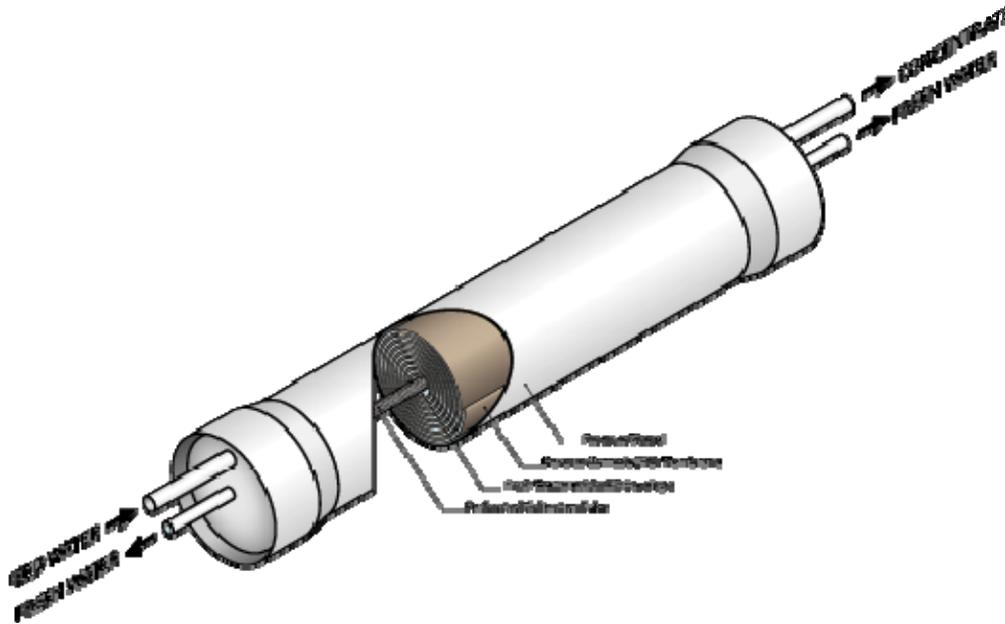
Figure 4 RO Membrane Modules are Generally “Spiral Wound” type. Feed spacer mesh forms a very narrow channel between membrane layers.
