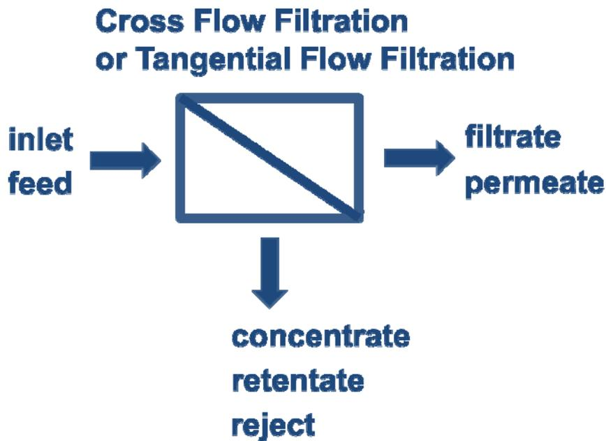
Figure 1: Cross Flow Filtration Schematic -An RO systems is a type of cross flow filtration system. Water flows tangentially along and across the RO membrane and helps to sweep the membrane clean, but pre-filtration is still needed.
