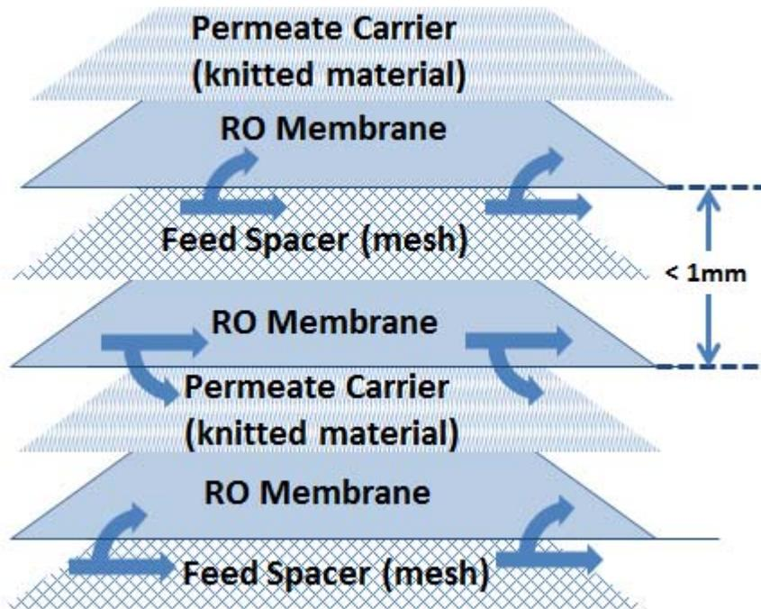
Figure 3 An RO filter module contains layers of feed spacer, RO membrane, and permeate carrier. The feed spacer creates a narrow channel subject to fouling.
