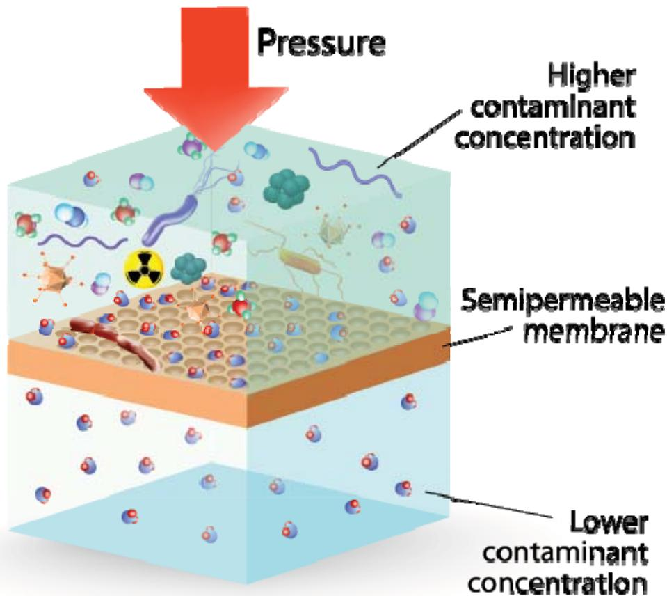
Figure 5- Reverse osmosis uses pressure to concentrate salts and dissolved molecules on the "concentrate" side of the membrane, and to push fresh water through to the "permeate" side of the RO membrane.
