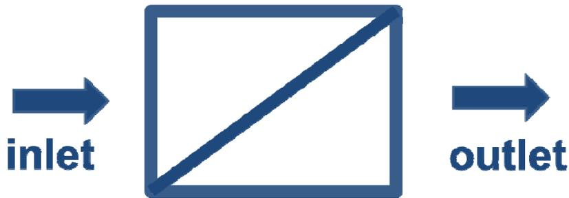
Figure 2 “Dead End Filtration” is commonly used for particulate filters, but is not used for Reverse Osmosis (RO). Dead end filtration has just one outlet, while RO filtration has two different kinds of “outlets”.
